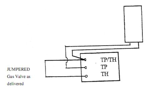
Remove factory jumper when installing remote control
